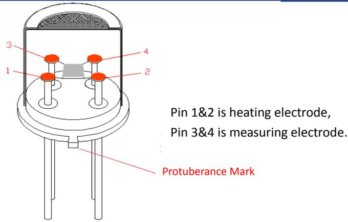
**Fig8.Pin Schematic Diagram**
