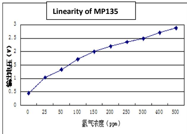
**Fig6. Linearity curve**
