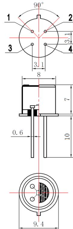
Fig1. Sensor Structure
